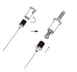
Loosen the top part of the hanging cable (C) and put the (A) screws in.
