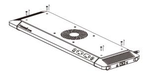
Remove the four corner screws from the AP700 using the hex wrench.
