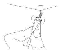
Step 2.2 Squeeze the sides of the toggle bolt (A), then insert into a pre-drilled hole. \*Hole Size - Min: 5/8"(16mm) / Max: 1"(25mm)
